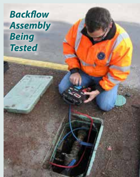
Reduced Pressure Backflow Assembly (RPBA) at Highline Headquarters
